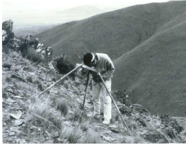
Figure 5 Taking photograph with stereophoto tripod with the stereophoto tripod set-up.
