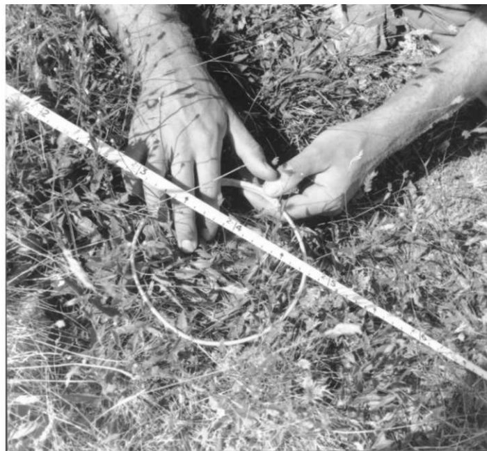
Figure 3 Delineating a specific subplot using the 15-cm diameter steel wire ring.
